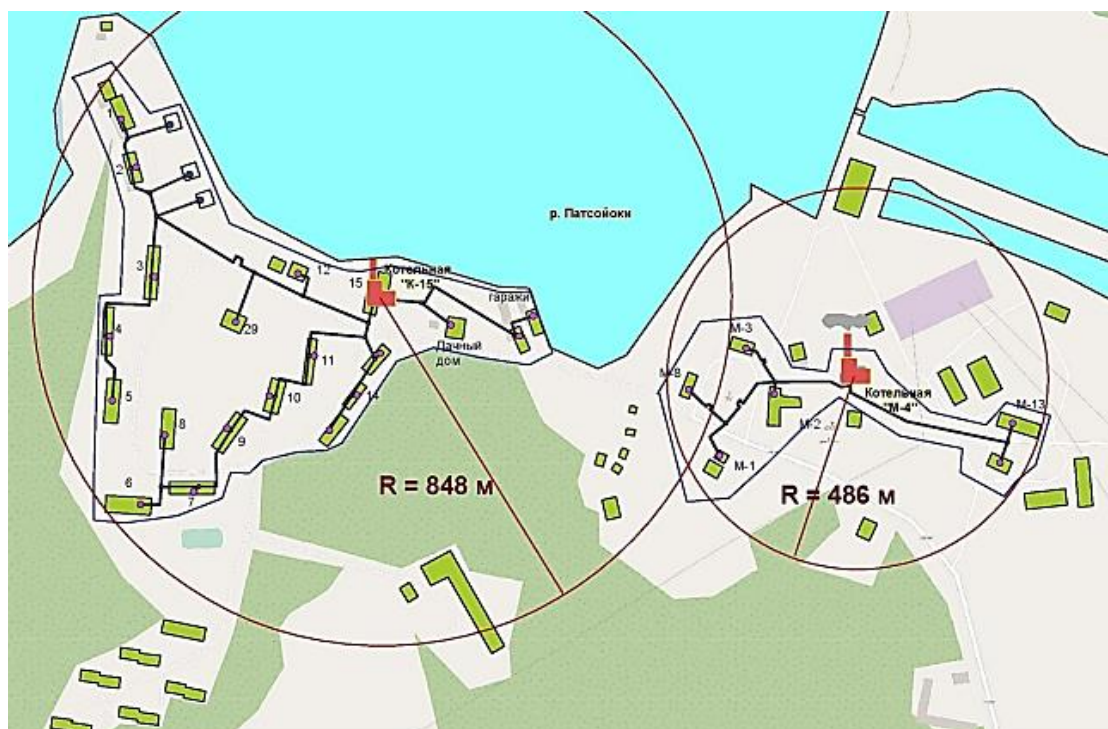
Рис. 5. Зоны действия электростанций н.п. Раякоски [11] Fig. 5. Operating zones of electric boiler houses in the village of Rayakoski [11]
